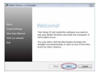
**Note:** If the Belkin Wireless Card Installer screen does not appear within 20 seconds, access your CD-ROM by double-clicking on the "My Computer" icon; then double-click on the CD-ROM drive into which the installation CD has been placed. If the Installer does not start automatically, double-click on the icon named "Installer.exe".
